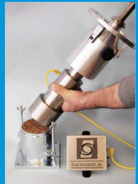
LWD-Lab unit is shown ready to test a sample in a Proctor mold.
