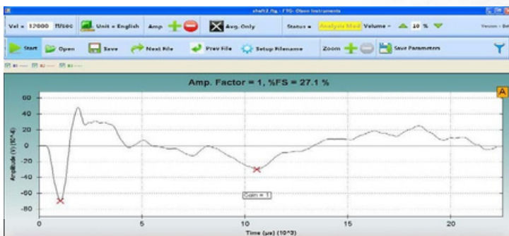
Olson's FTG Software showing sonic echo waveform
