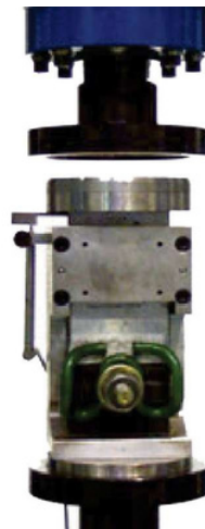
Fatigue tests under lateral loads for sleepers light fastening plates
