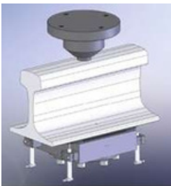
Rigidity test over elastic plates for a high speed rail
