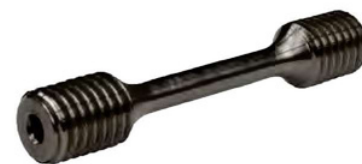
Typical steel specimen for creep test
